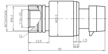
The RS124B-230 series adopts diffused silicon or ceramic piezoresistive sensor chip, with compact configuration, easy to install, and special valve pin design for lead pressure port, perfect electrical performance and long-term stability make it the idea choice for the air-condition and compressor pressure measuring and controlling.
